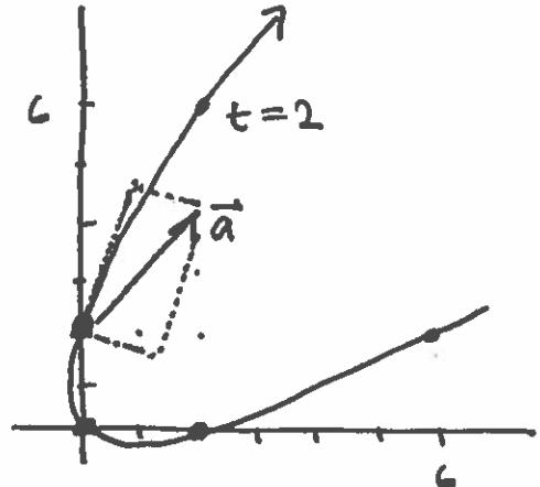
Decompose  $\vec{a}(t) = \left( \begin{array}{c} \text{Some scalar changing over time} \\ \text{over time} \end{array} \right) \cdot \vec{T}(t) + \left( \begin{array}{c} \text{some scalar changing over time} \\ \text{over time} \end{array} \right) \cdot \vec{N}(t)$
