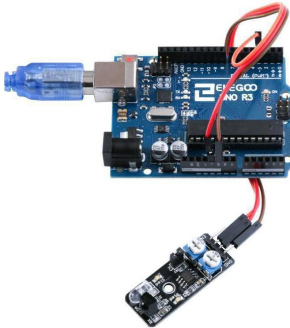
Here we use the obstacle avoidance module and a digital interface, built-in 13 LED build a simple circuit, making avoidance warning lamp, the obstacle avoidance Sensor Access Digital 3 interface, when obstacle avoidance sensor senses a signal, LED light, and vice versa off.
