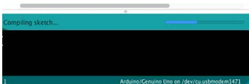
Next, the status will change to 'Uploading'. At this point, the LEDs on the Arduino should start to flicker as the sketch is transferred.
