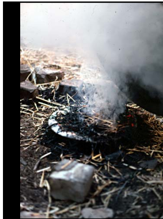
The reduction area is covered to extinguish the flame and cause it to smolder, creating smoke. This process forces carbon molecules into the exposed clay body and effect any glaze with the bombardment of carbon.
