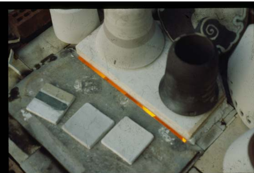
The chamber is gradually heated to approx 1900° F. Usually in three increments. This process may take as little as 30 minutes.
