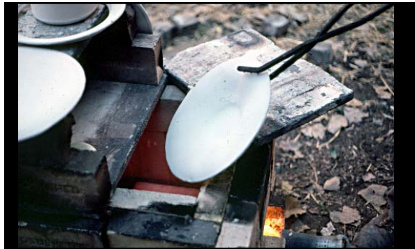
Using tongs the pot is placed in the heated fire chamber – approx 1700° F
