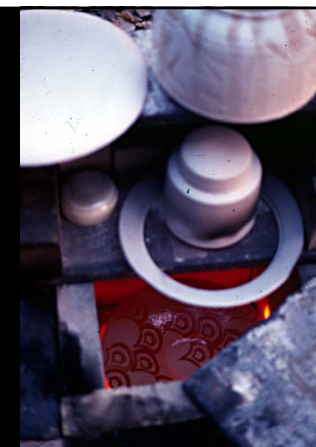
Most raku glazes mature at approx 1900° F. Notice the shine on the surface of the pot inside the kiln. A sign that it is ready to be removed.
