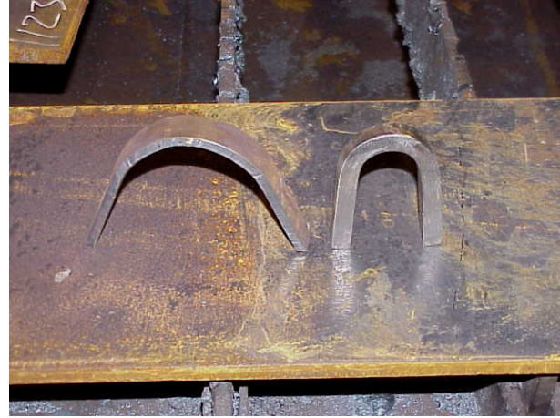
The bend samples shown above differ in the radius that they were bent. This is a requirement set forth by the code or standard that is being used.
