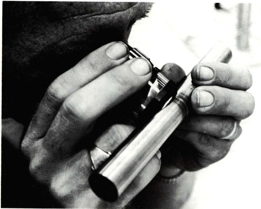
Inspector examines weld surface through a magnifying lens to make sure that appearance complies with code requirements.
